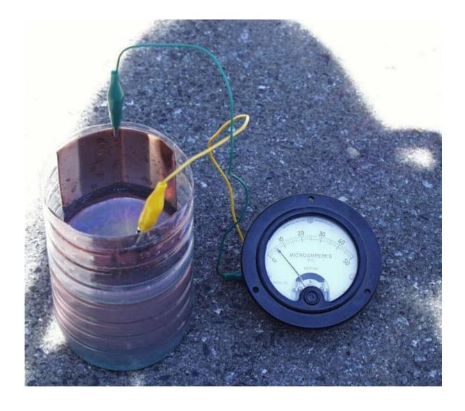
The photo above shows the solar cell in my shadow as I took the picture. Notice that the meter is reading about 6 microamps of current.
