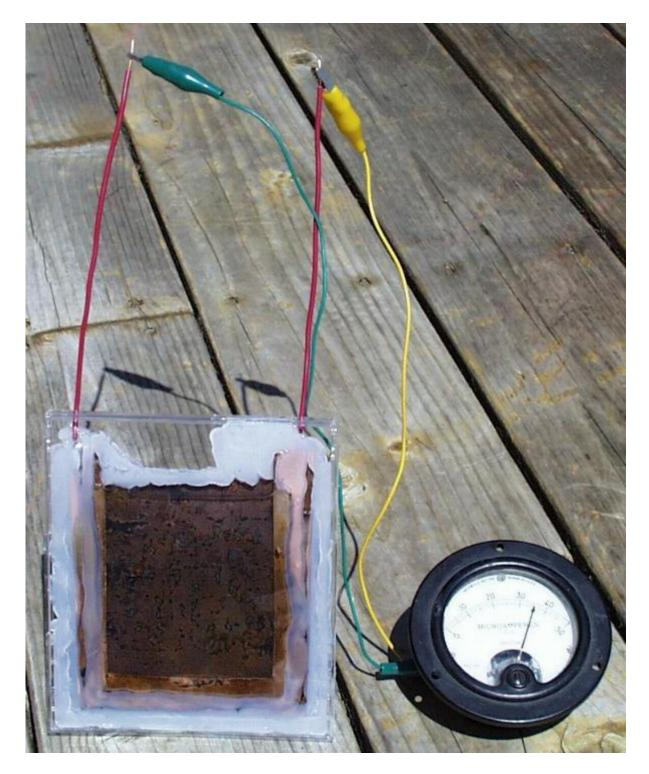
In the photo above you can see the flat panel solar cell in action in the bright sun. It is delivering about 36 microamperes of current. You can also see the extra bead of glue around the edges of the plates, and filling the top of the funnel.
