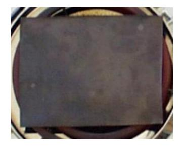
When the burner is glowing red-hot, the sheet of copper will be coated with a black cupric oxide coat. Let it cook for a half an hour, so the black coating will be thick. This is important, since a thick coating will flake off nicely, while a thin coat will stay stuck to the copper.
