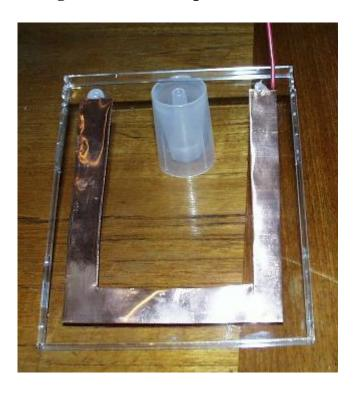
The photo below shows the front side of the solar cell (the side that will face the sun) at this point in the construction. Notice that the silicone glue does not completely cover the copper, since some of the copper must eventually be in contact with the saltwater.
