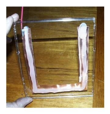
The next step is to lay a good size bead of glue onto the U shaped clean copper plate. This layer will act as an insulator between the clean copper plate and the cuprous oxide plate, and must be thick enough to leave some room for the saltwater. Again, not all of the copper is covered, so there will be plenty of copper in contact with the saltwater.
