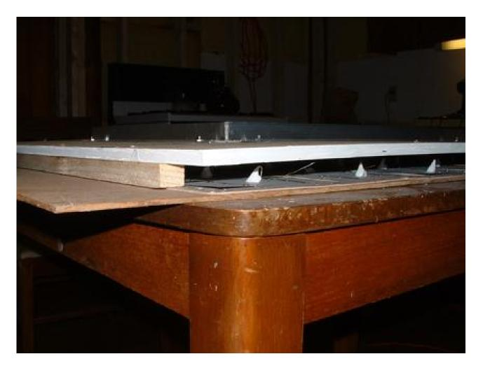
The next step is to flip the rig over. This can be tricky, but I find using two small C-clamps opposite each other holds the backing and the jig together just enough to let me flip it over without any of the cells moving on me. Here is the new panel with the jig removed.
