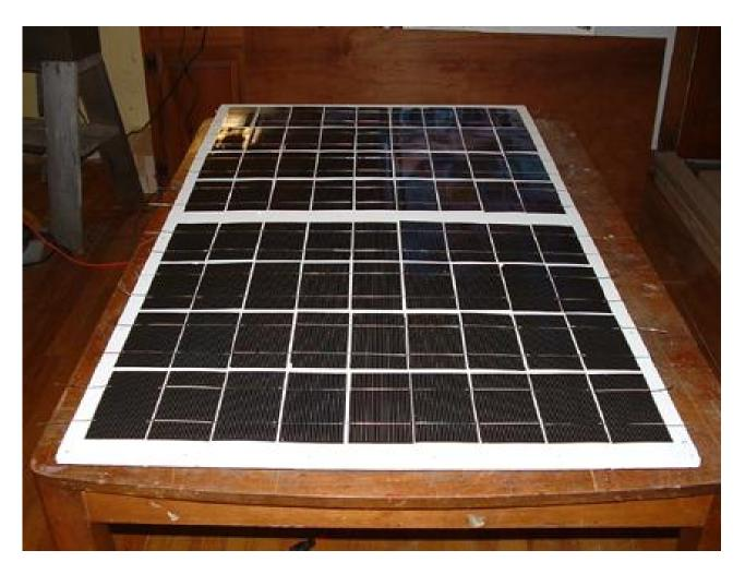
Power is brought to the back of the panel using bolts counter sunk into the plywood. The copper strip is .015 copper sheet purchased on-line and cut up into strips.
