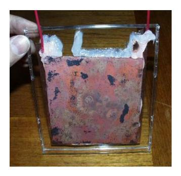
The photo below shows the front side of the solar cell (the side that will face the sun) at this point in the construction. Note that I added extra glue to form a funnel at the top to allow the saltwater to be added.
