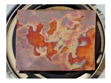
As the copper gets hotter, the colors are replaced with a black coating of cupric oxide. This is not the oxide we want, but it will flake off later, showing the reds, oranges, pinks, and purples of the cuprous oxide layer underneath.
