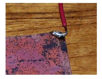
The positive plate is a U shaped piece cut from the copper sheeting, a little bit larger than the cuprous oxide plate, with the cutout portion
