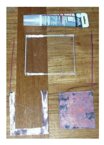
The first step is to make a cuprous oxide plate like we did in the first solar cell. This time I sanded one corner clean all the way down to the shiny copper, and soldered an insulated copper wire to it for the negative lead.
