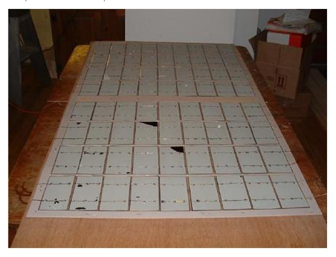
Here the cells are all soldered and a dab of silicone caulk is placed on each one.
