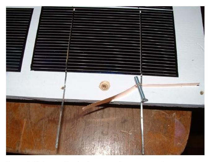
The terminal bolts are soldered to the copper strip to ensure a good connection. The copper is also used to string the rows of cells together at the ends.
