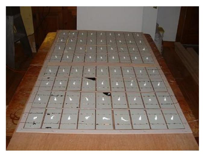
I used 1/2 inch plywood for my backing. It sits atop spacers as I align it with marks on my jig. When it is in the right position I remove the spacers and let it press into the silicone. You may be able to make out the  $1 \times 1 \times 1/16$  inch aluminum angle stock that's bolted to the upper face of the plywood. The angle stock is bent into an 'L' shape and two of them are set to form a rectangular shape and bolted down. The metal adds a great deal of stiffness to the plywood.
