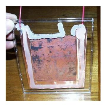
Not shown in the photo is a generous extra bead of glue all around the outside of the plates, to ensure that no saltwater will leak out. Allow the glue to cure before going on to the next step.
